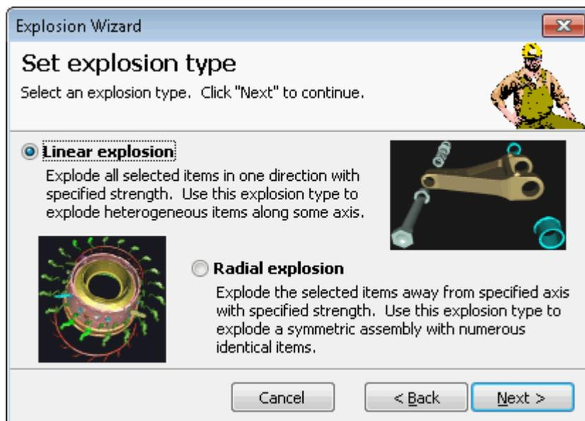
**Linear explosion** explodes the selected Items along the specified axis with the specified strength. The selected Items are placed equidistantly from each other along the chosen axis (see the figure below).
